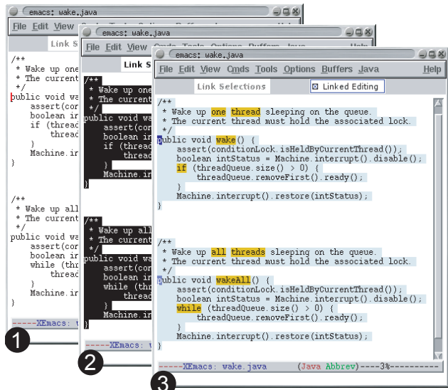
Figure 1. (1) Before linking two similar Java methods in Codelink. (2) After selecting the methods. (3) After linking the methods.
